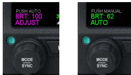
Figure 8 - Lighting control adjustment
