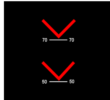
Figure 13 - Excessive Pitch Up
