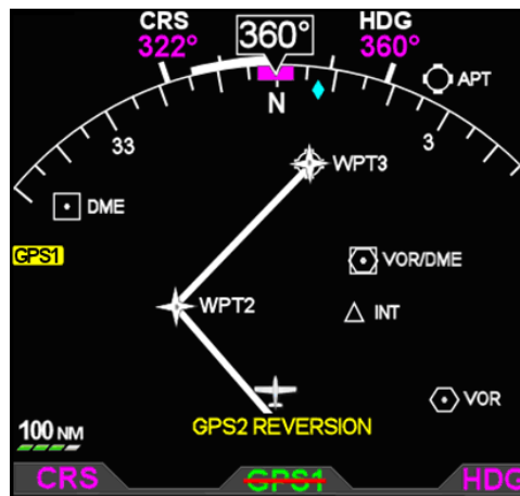
Figure 35 – GPS1 Failure, Reversionary Navigation
