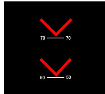
Figure 13 - Excessive Pitch Up
