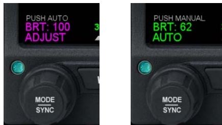
Figure 8 - Lighting control adjustment
