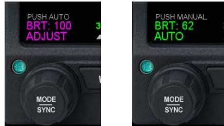
Figure 6 - Lighting control adjustment
